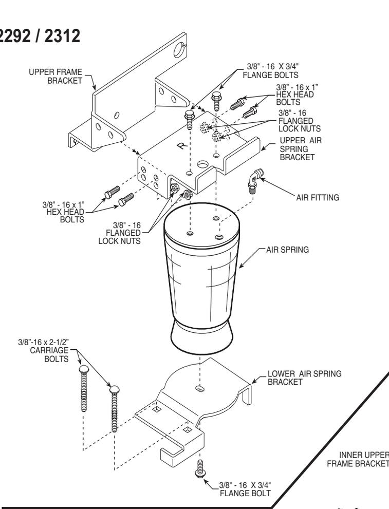
NOTE: Both illustrations are of the right side, of the van. Refer to Step 3 for the proper lower bracket alignment.
