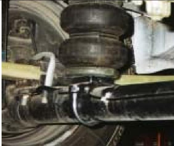
Route the longer air tube from the airspring along the underneath of the vehicle to the other side and connect with a Tee fitting to the tube from the other airspring.
