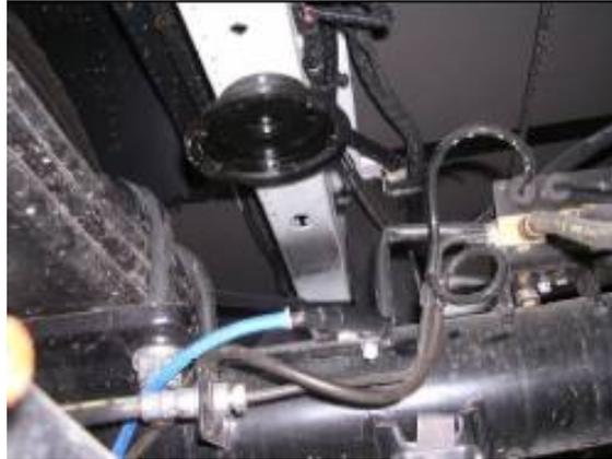
The top of the air spring has two studs and an air entrance hole. Attach the upper bracket to the top of the bellows using the 3/8" hex nuts and spring washers provided making sure that the air entrance hole is exposed in the bracket opening.
