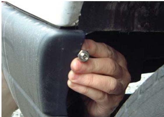
Cut a generous length of air tubing to reach from the inflation valve to the top of the nearest airspring, following the line of the inner wheel arch and across to the top of the airspring, with sufficient slack to allow suspension movement. Insert one end of this tube into the air fitting in the airspring.
