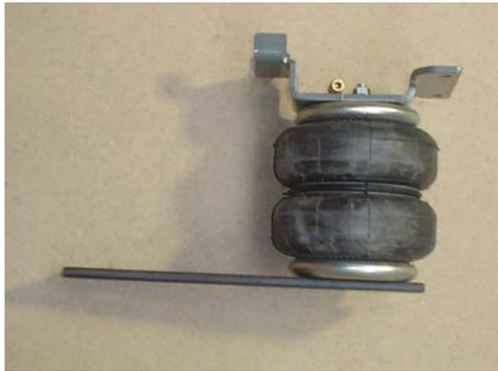
Raise the body of the vehicle until the wheels are approximately 50 mm above the ground, to allow space to insert the spring assemblies, which are mounted behind the rear axle. Support the rear axle with a jack.
