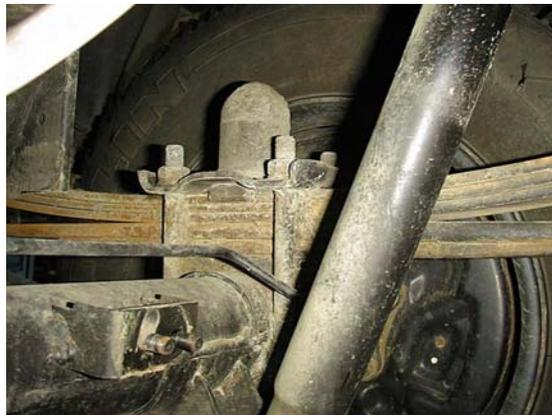
Loosen the four original U bolt nuts each side. Place the assembled airsprings between the chassis and the axle, and slide the extended side of the bottom bracket underneath the clamp plate until the spring centre pin is located in the slot on the bracket.
