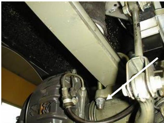
In order to mount the lower bracket the U-bolt must be used.
