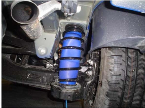
With the tubing routed from the air spring to the location of the inflation valve. Use the nylon ties supplied to secure the air line tubing to the vehicle as shown. Be careful to avoid heat and sharp edges when fastening the tubing to the vehicle. Route the tubing away from the exhaust system.
